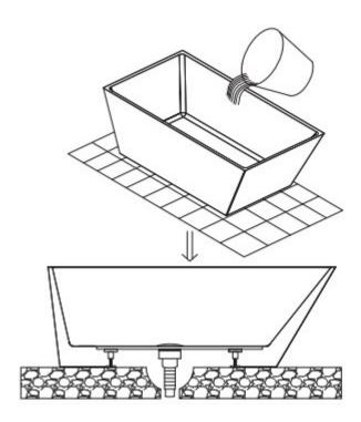
2-5. Apply a thick layer of silicon sealant around the bath outline allow it set 24 hours. This installation guide, the installation of waste connection should be only
